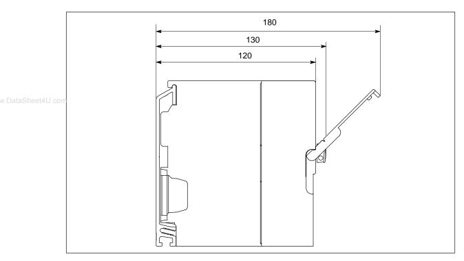
Figure E-5 shows the dimensioned drawing of the CPU 314 IFM, side view.
