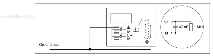
Figure 4-4 S7-300 Configuration with Ungrounded Reference Potential
