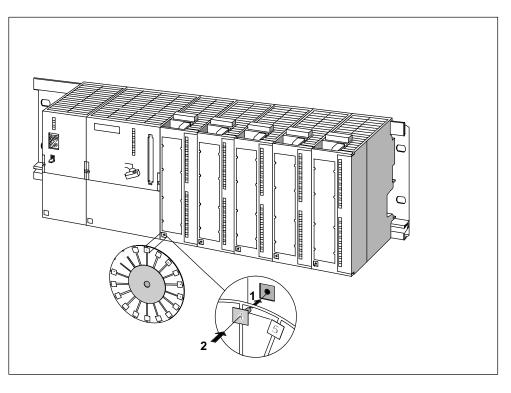
Figure 2-8 Applying Slot Numbers to the Modules
