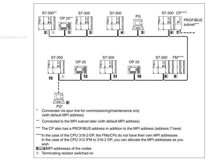
Figure 5-4 Example of an MPI Subnet
