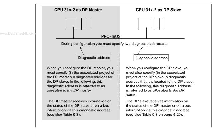
Figure 9-3 Diagnostic Addresses for DP Master and DP Slave
