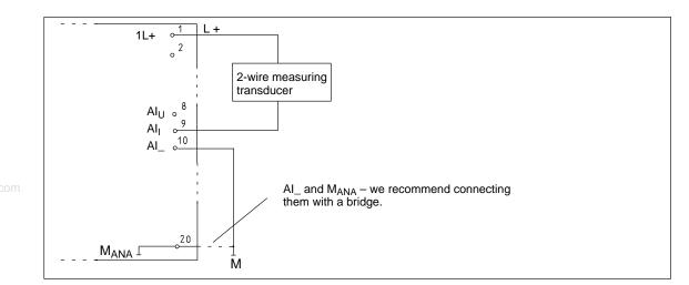
Figure 8-13 Wiring the Analog Inputs of the CPU 314 IFM with a 2-Wire Measuring Transducer
