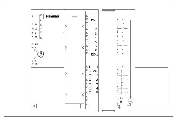
Figure 8-6 Terminal Assignment Diagram of the CPU 312 IFM
