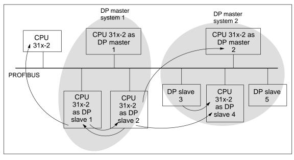
Figure 9-14 Direct Communication with CPU 31x-2
