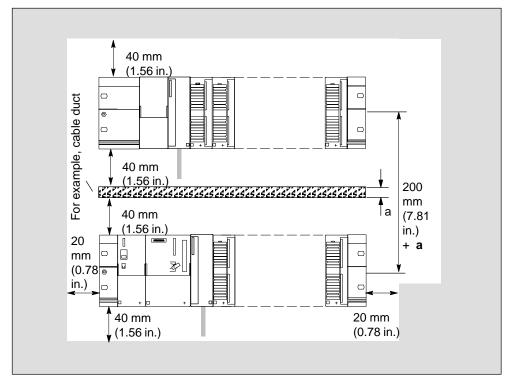
Figure 2-2 Clearance Measurements for an S7-300 Installation
