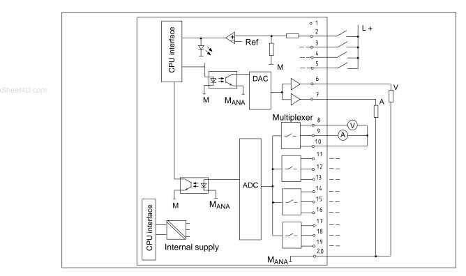
Figures 8-11 and 8-12 show the basic circuit diagrams for the integrated inputs/outputs of the CPU 314 IFM.
