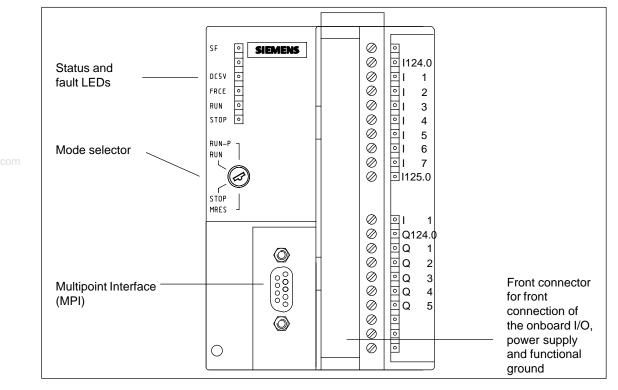
Figure 8-5 Front View of the CPU 312 IFM
