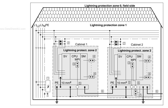
Figure 4-11 Example of the Interconnection of Networked S7-300s
