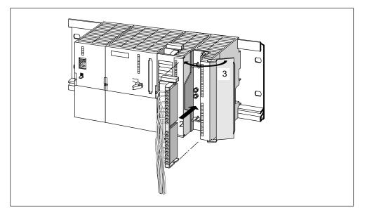
Figure 7-5 Plugging In the Front Connector
