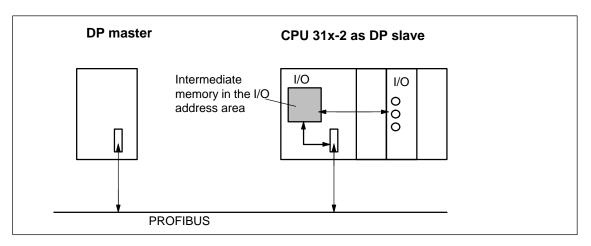
Figure 9-4 Intermediate Memory in the CPU 31x-2 as DP Slave
