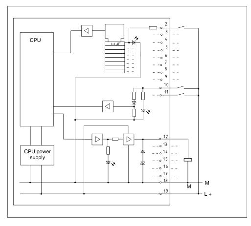
Figure 8-7 Basic Circuit Diagram of the CPU 312 IFM
