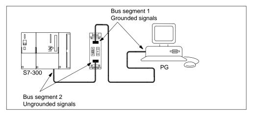
Figure 6-6 Programming Device Connected to an Ungrounded S7-300
