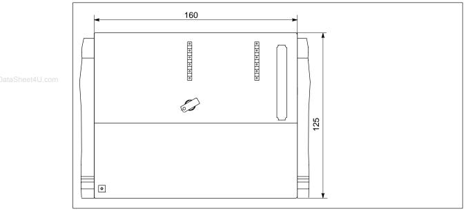
Figure E-3 Dimensioned Drawing of the CPU 318-2
