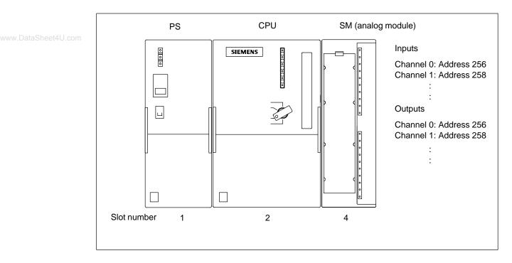
Figure 3-4 Addresses of the Inputs and Outputs of the Analog Module in Slot 4
