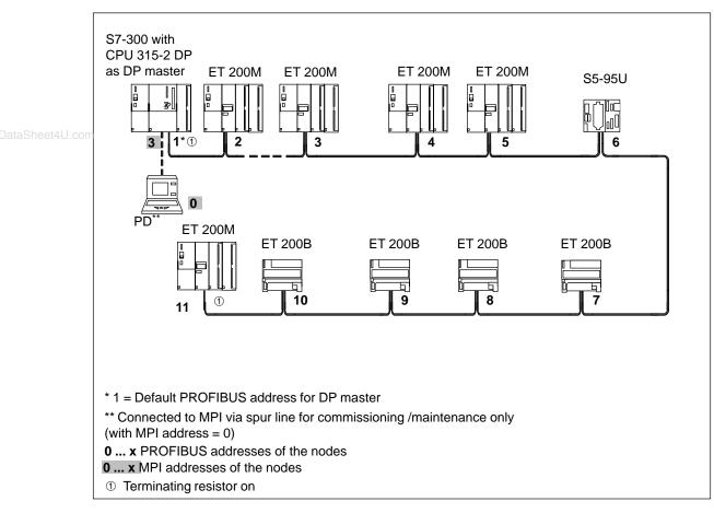
Figure 5-5 Example of a PROFIBUS Subnet
