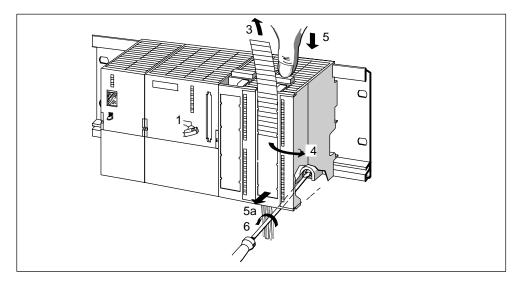
Figure 7-2 Unlocking the Front Connector and Detaching the Module from the Rail
