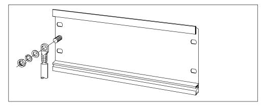
Figure 2-6 Connecting the Protective Conductor to the Rail
