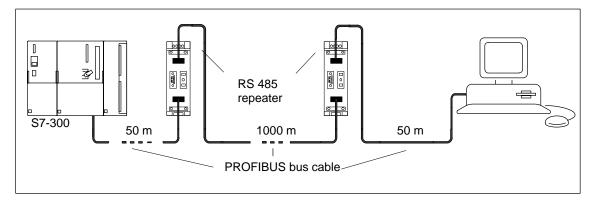
Figure 5-7 Maximum Cable Length Between Two RS 485 Repeaters
