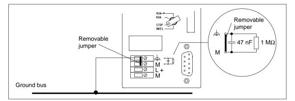
Figure 4-3 S7-300 Configuration with Grounded Reference Potential
