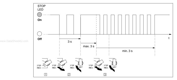
Figure 6-7 Switching Sequence for the Mode Selector for Resetting the CPU
