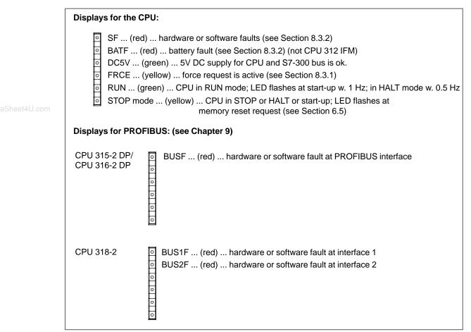
Figure 8-2 Status and Fault Displays of the CPUs
