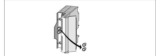
Figure 7-3 Removing the Front Connector Coding Key
