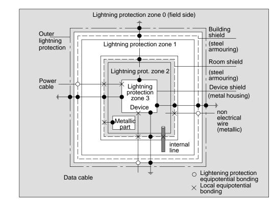
Figure 4-10 shows a schematic of the lightning protection zone concept for a free-standing building.
