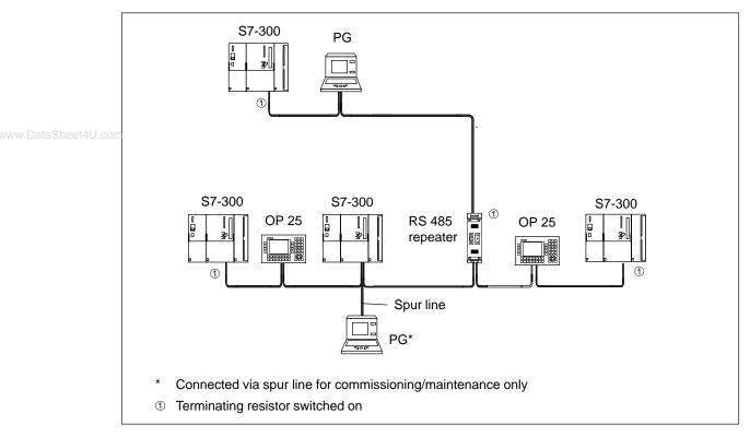
Figure 5-3 Connecting Terminating Resistors in an MPI Subnet
