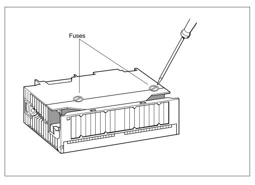
Figure 7-6 Location of the Fuses on Digital Output Modules
