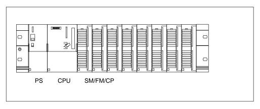
Figure 2-3 Module Arrangement for an S7-300 Programmable Controller Mounted on One Rack
