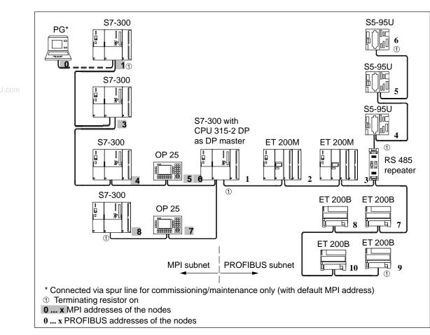
Figure 5-6 shows an MPI subnet with an integrated CPU 315-2 DP that is also operating as a DP master in a PROFIBUS subnet.
