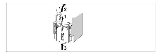
Figure 5-10 Removing the Slide on the RS 485 Repeater
