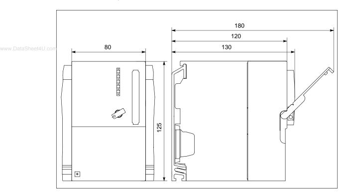
Figure E-2 Dimensioned Drawing of the CPU 313/314/315/315-2 DP/316-2 DP
