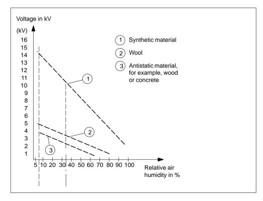
Figure F-1 Electrostatic Voltages which can Build up on a Person
