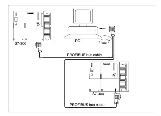
Figure 6-4 Connecting a Programming Device to Several S7-300s
