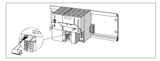
Figure 6-2 Inserting a Backup Battery in the CPUs 313/314
