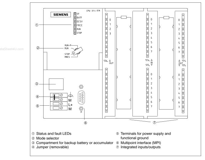
Figure 8-9 Front View of the CPU 314 IFM
