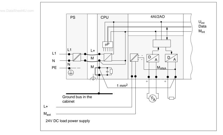
Figure 4-6 Potentials in a Configuration with the Non-Isolated SM 334 Analog Input/Output Module; AI 4/AO 2  $\times$  8/8Bit
