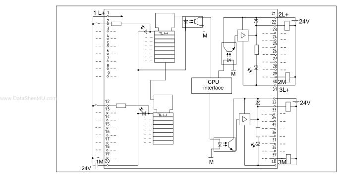
Figure 8-12 Basic Circuit Diagram of the CPU 314 IFM (Digital Inputs/Outputs)
