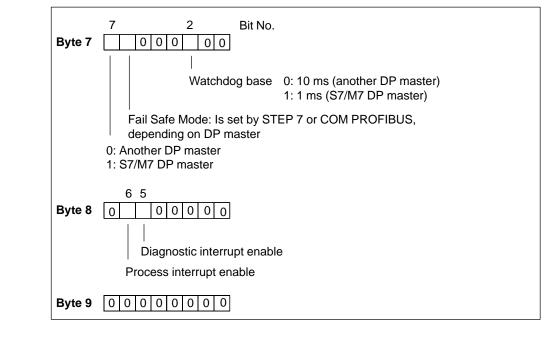
Figure 9-11 Parameters for the CPU 31x-2
