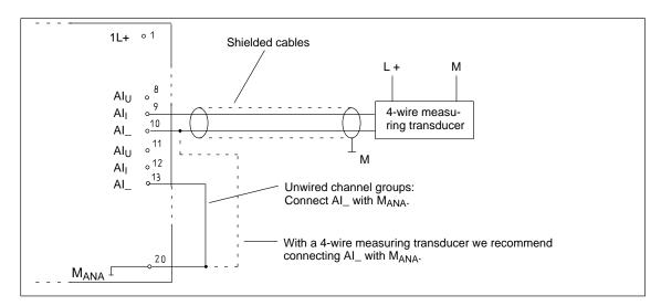
Figure 8-14 Wiring the Analog Inputs of the CPU 314 IFM with a 4-Wire Measuring Transducer
