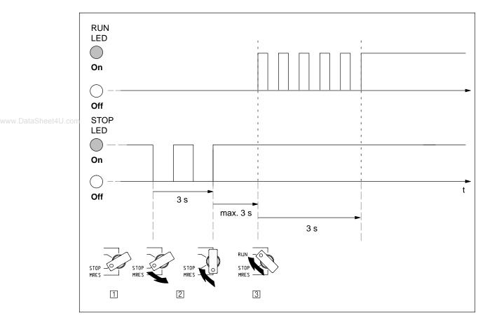
Figure 6-8 Switching Sequence for the Mode Selector for Cold Start (CPU 318-2 Only)
