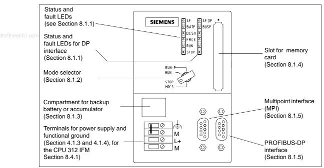
Figure 8-1 Control and Display Elements of the CPUs
