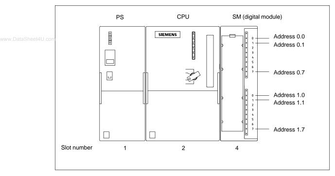
Figure 3-3 Addresses of the Inputs and Outputs of the Digital Module in Slot 4
