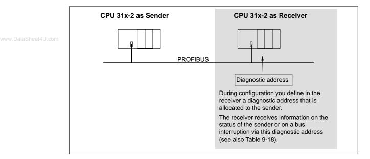
Figure 9-15 Diagnostic Address for the Receiver During Direct Communication
