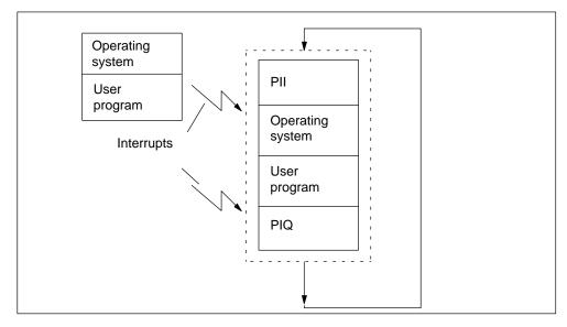
Figure 10-1 Component Parts of the Cycle Time
