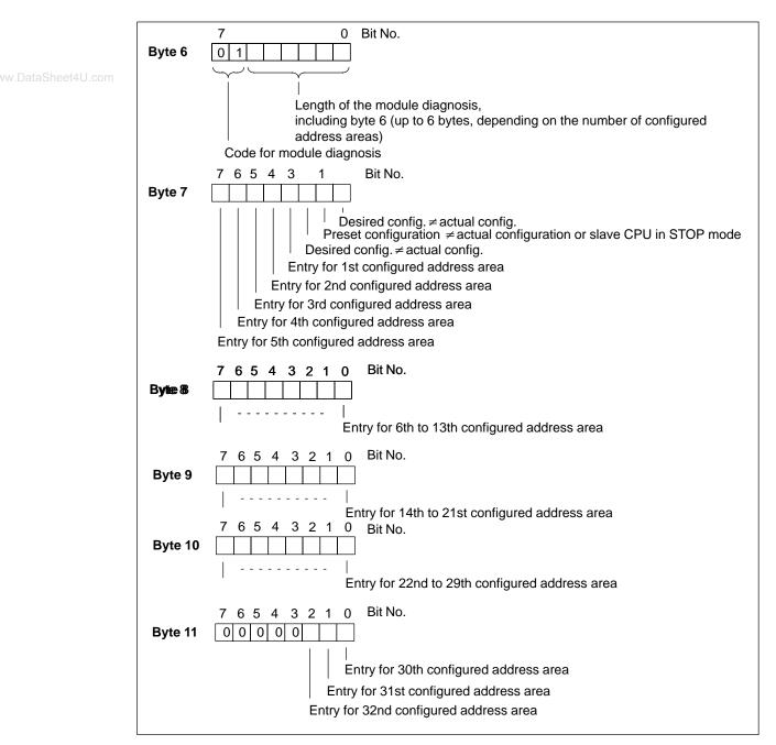
Figure 9-7 Structure of the Module Diagnosis of the CPU 31x-2
