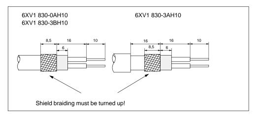
Figure 5-11 Lengths of the Stripped Insulation for Connection to the RS 485 Repeater
