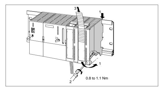
Figure 7-4 Installing a New Module
