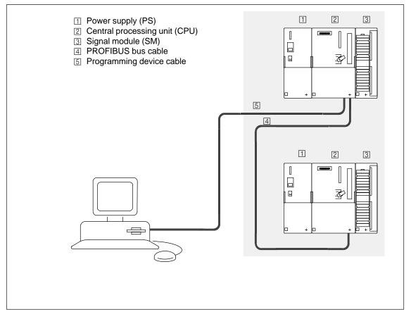
Figure 1-1 Components of an S7-300
