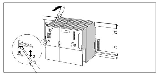
Figure 4-13 Setting the Mains Voltage for the PS 307
