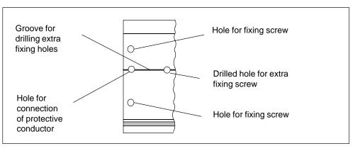
5. Tighten the M6 screw to fix the protective conductor.
