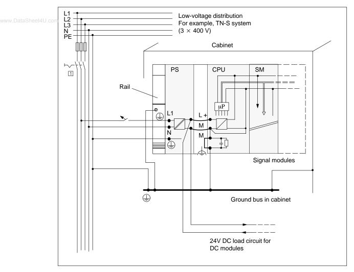
Figure 4-2 Signal Modules Powered from the PS 307
