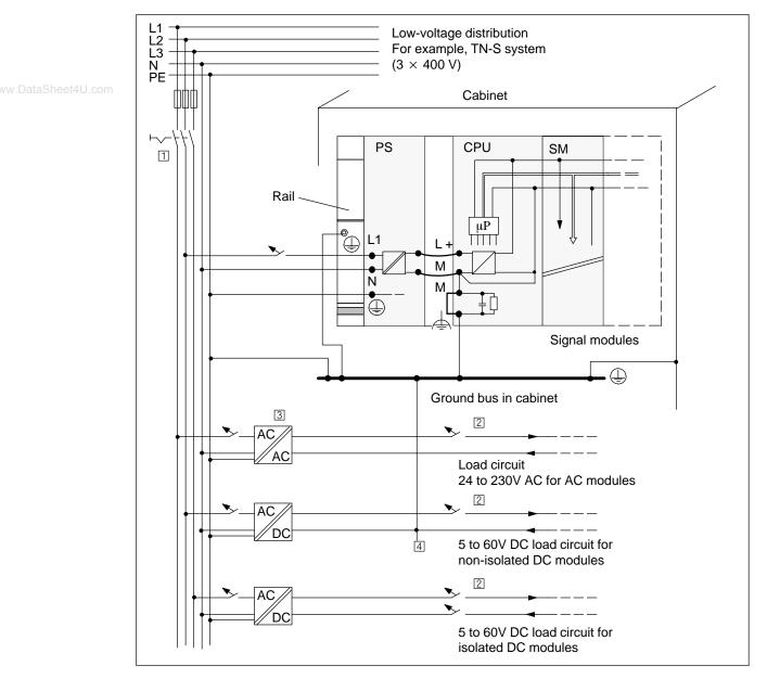
Figure 4-1 Signal Modules Operated on a Grounded Incoming Supply
