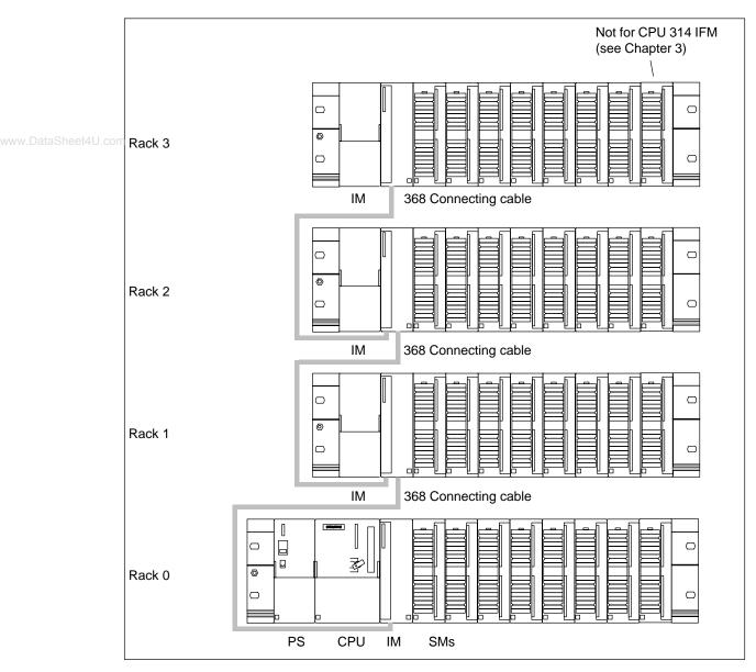
Figure 2-4 Arrangement of Modules in a Four-Rack S7-300 Configuration
