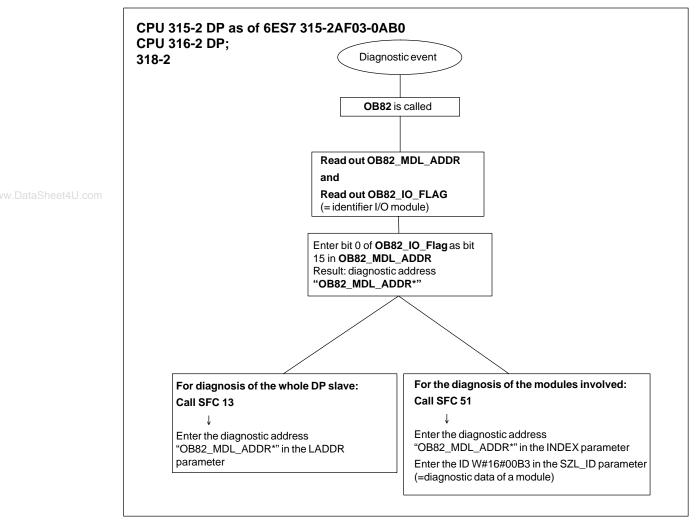
Figure 9-2 Diagnostics with CPU 31x-2 (315-2 DP as of 315-2AF03)
