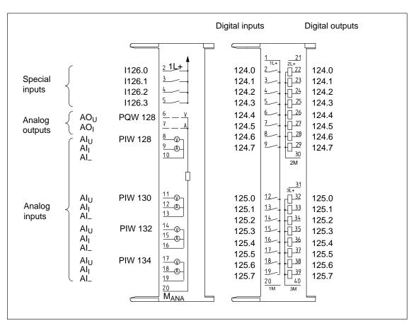
Figure 8-10 Terminal Assignment Diagram of the CPU 314 IFM
