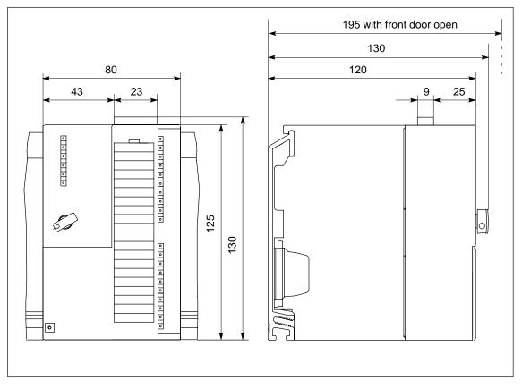
Figure E-1 shows the dimensioned drawing of the CPU 312 IFM.
